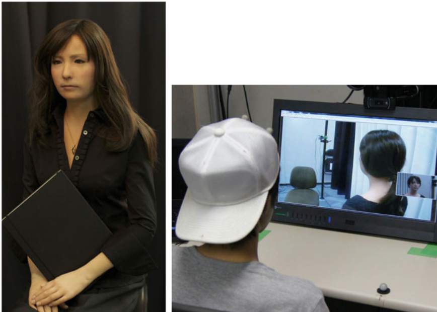
Fig. 20.1 Teleoperated android robot Geminoid F (left) and its teleoperation interface (right). In the teleoperation monitor, the operator can see both the interlocutor (near first-person view, main screen) and the face of the geminoid (second-person view, subscreen)
