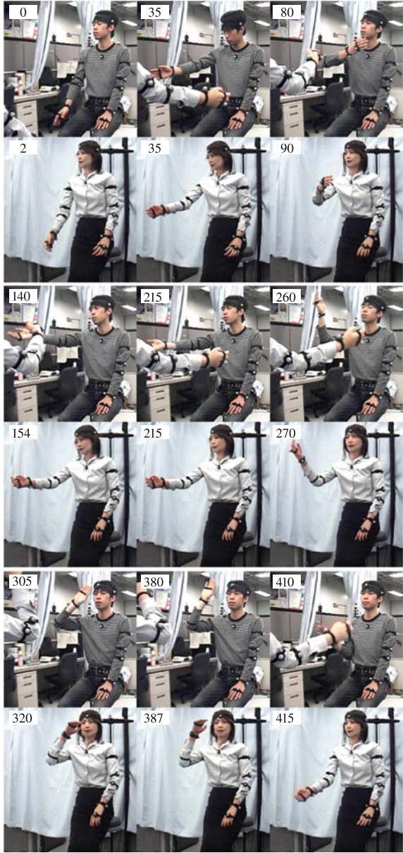
Fig. 4.11 Generated android motion compared to the performer's motion. The numbers represent steps
