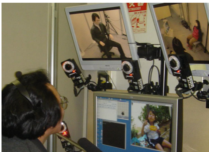
Fig. 11.2 Geminoid teleoperation console
