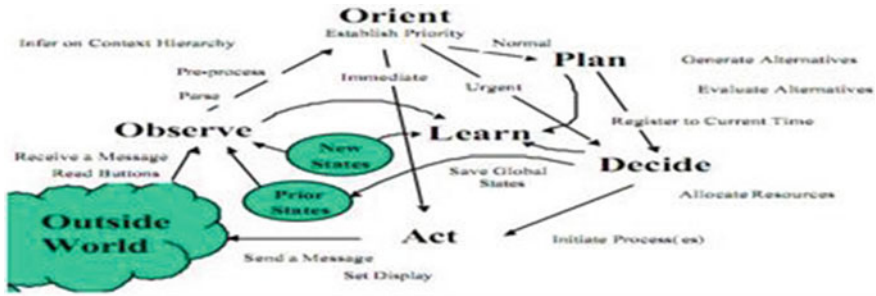
Fig. 1 Cognitive radio recognition cycle [1]
