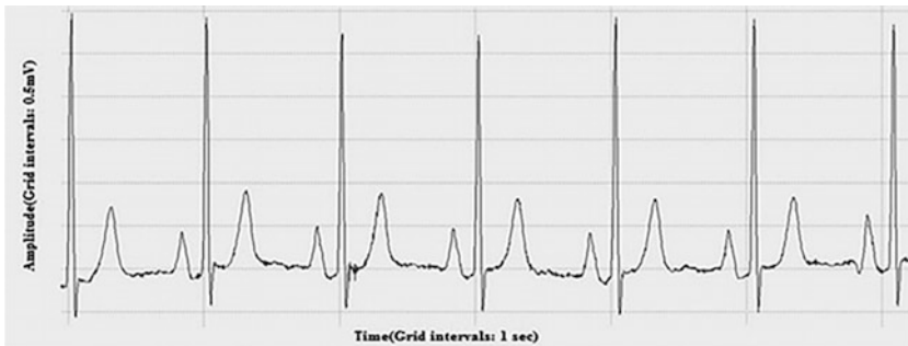
Fig. 3 Denoised ECG signal using an FIR equiripple filter
