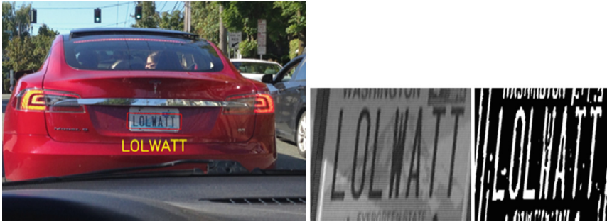
Fig. 10. (a) Image obtained through other vehicles mirror, the input image finds exact match of the detected license plate (b) extracted license plate and threshold output.
