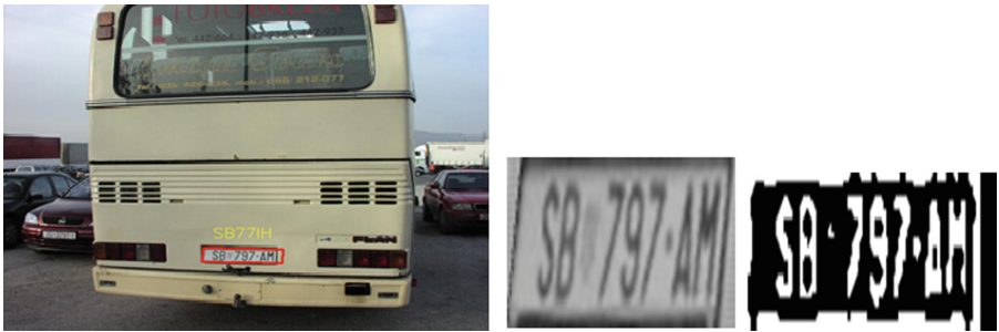
Fig. 11. Image of a tourist bus with relevant output of license plate number
