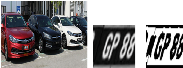
Fig. 8. (a) parking slot image. (b) Extracted license plate and threshold output.
