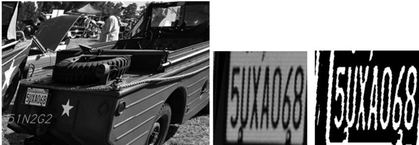
Fig. 9. (a) Image of a military vehicle produces best result in spite of tilted characters (b) extracted license plate and threshold output.
