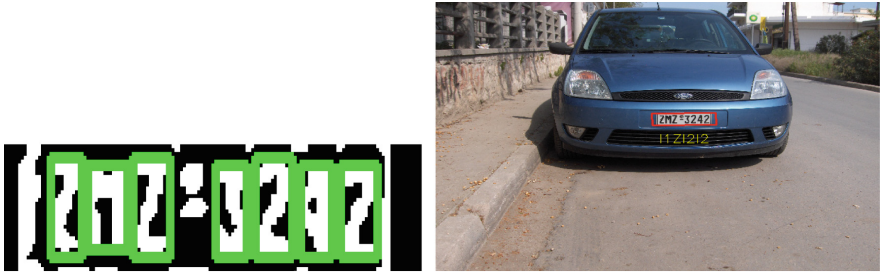
(a) the output KNN training of obtained plate (b) This is the final output with nearest match
