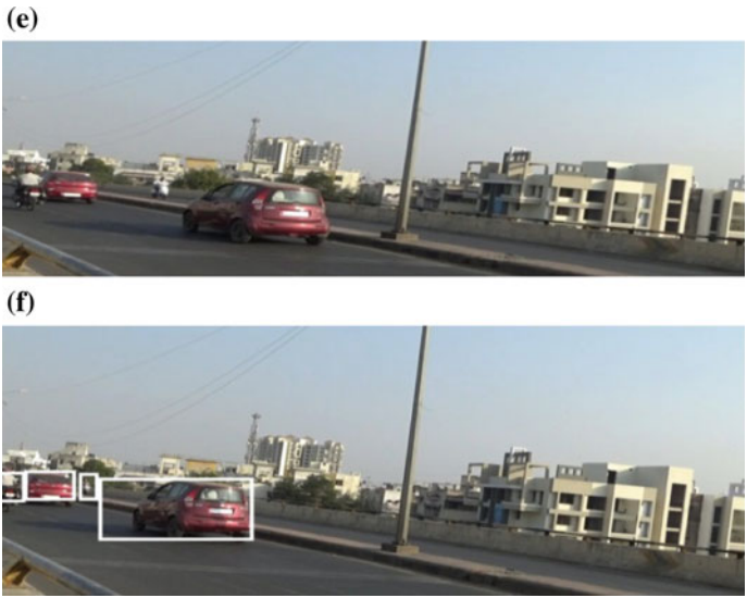
Fig. 8 Multiple object detection. e Original frame (161st of highway_traffic.mp4). f Detected frame using variance-based method
