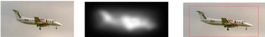
Fig. 2 Starting from left, original image followed by the saliency map and original image with bounding box
