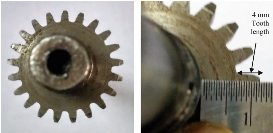
Fig. 2 Good gear tooth
