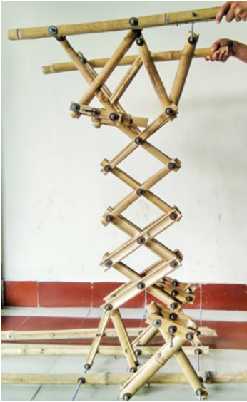
(a) Parallel-plane scissor mechanism made by bamboo pieces
