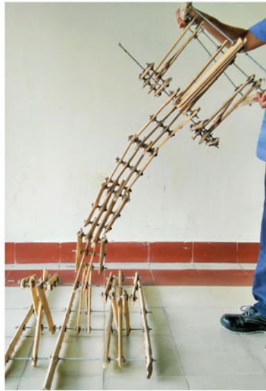
(b) Lateral sway in parallel-plane scissor mechanism
