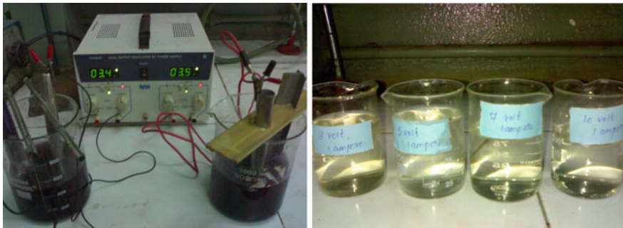
Fig. 8 Laboratory-scale electrocoagulation process
