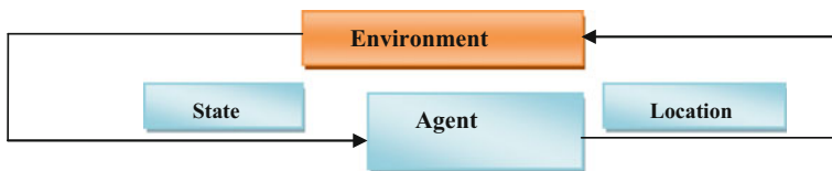
Fig. 3 Block diagram for process of reinforcement learning [1]
