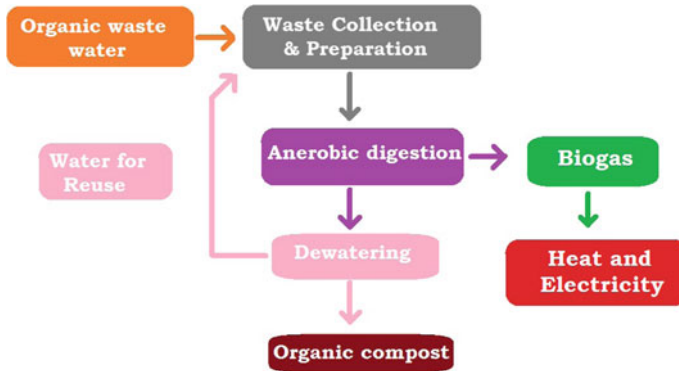
Fig. 5 Anaerobic wastewater treatment
