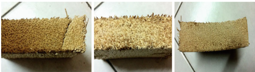
Fig. 4 Drying defect of end check, honeycomb and deformation
