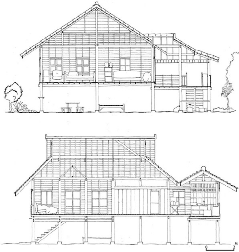
Fig. 8.2 Sections of a raised-floor house
