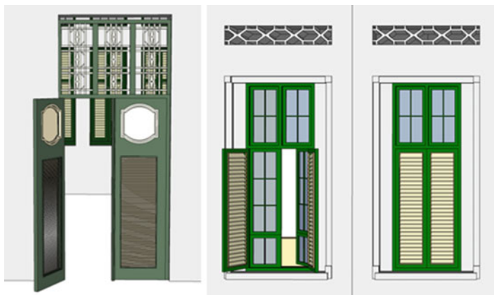
Fig. 2.3 Louver door and ventilation openings above windows/doors
