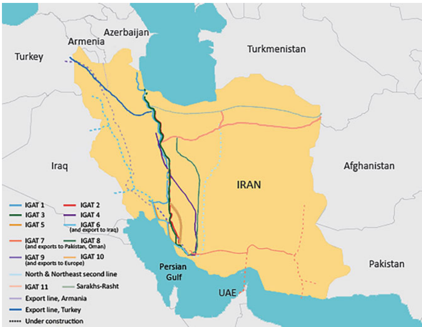
Fig. 12 Iran Gas Trunk-line
