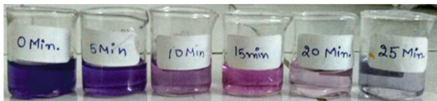
Fig. 8 EBT solutions before and after sorption on aminosilane modified magnetic nanosilica
