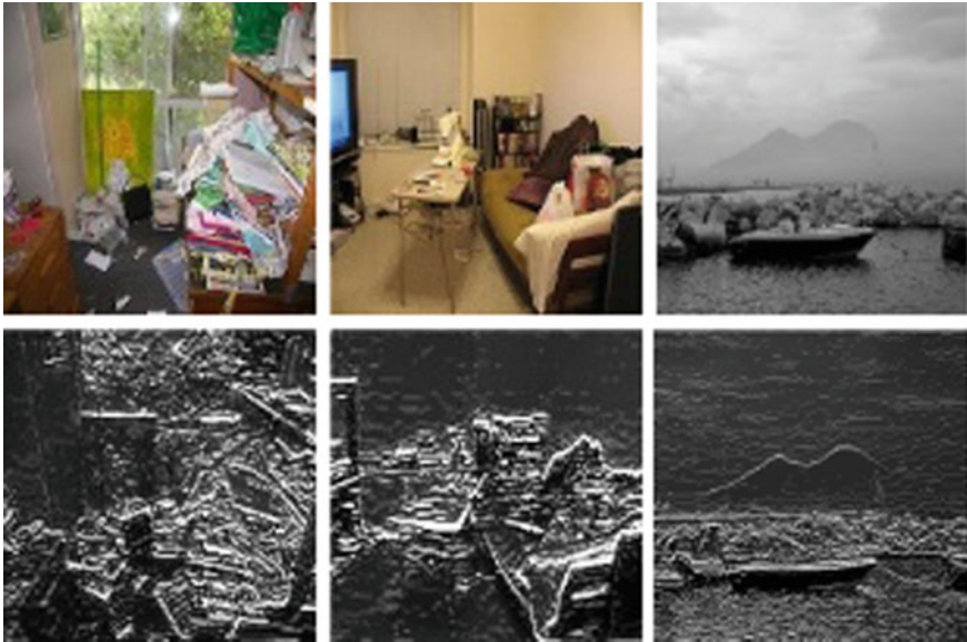
Fig. 2 The first set of images are the input images from ImageNet dataset, and the second set of images represent enhanced output due to the iterative Sobel filter based on entropy
