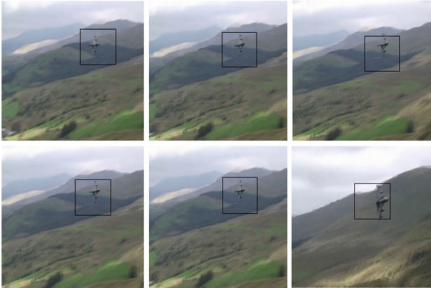
Fig. 5 Sample video-1 object tracking simulation results using SIFT
