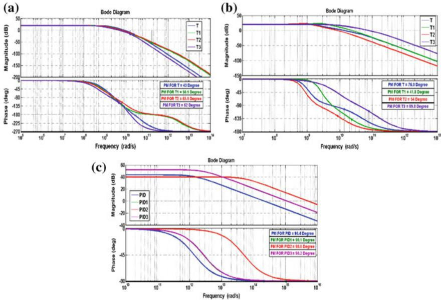
**Fig. 5.** **a** Bode responses of the simulated second-order LF model. **b** Bode responses of the simulated third-order LF model. **c** Bode responses of the simulated PID controller model
