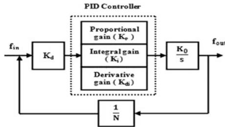
Fig. 2. Functional block diagram of the model
