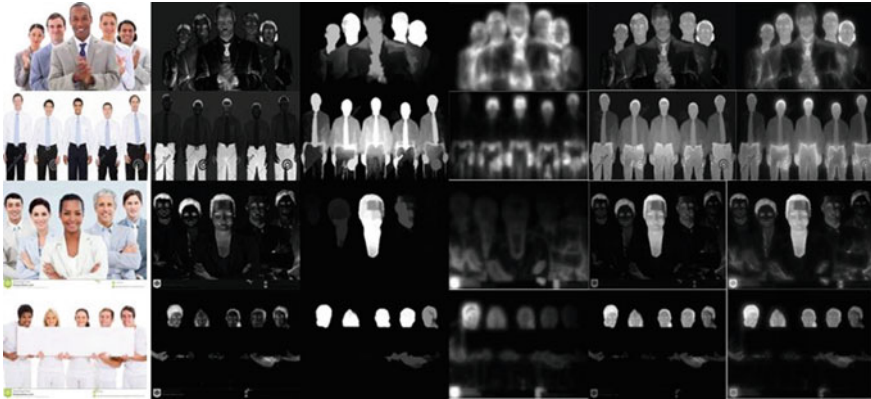
Fig. 3. Row wise—first column: input image, second column: saliency map using [17], third column: saliency map using [18], fourth column: saliency map using [19], fifth column: saliency map after fusing methods [17, 18], sixth column: proposed master saliency map after fusing methods [17–19]
