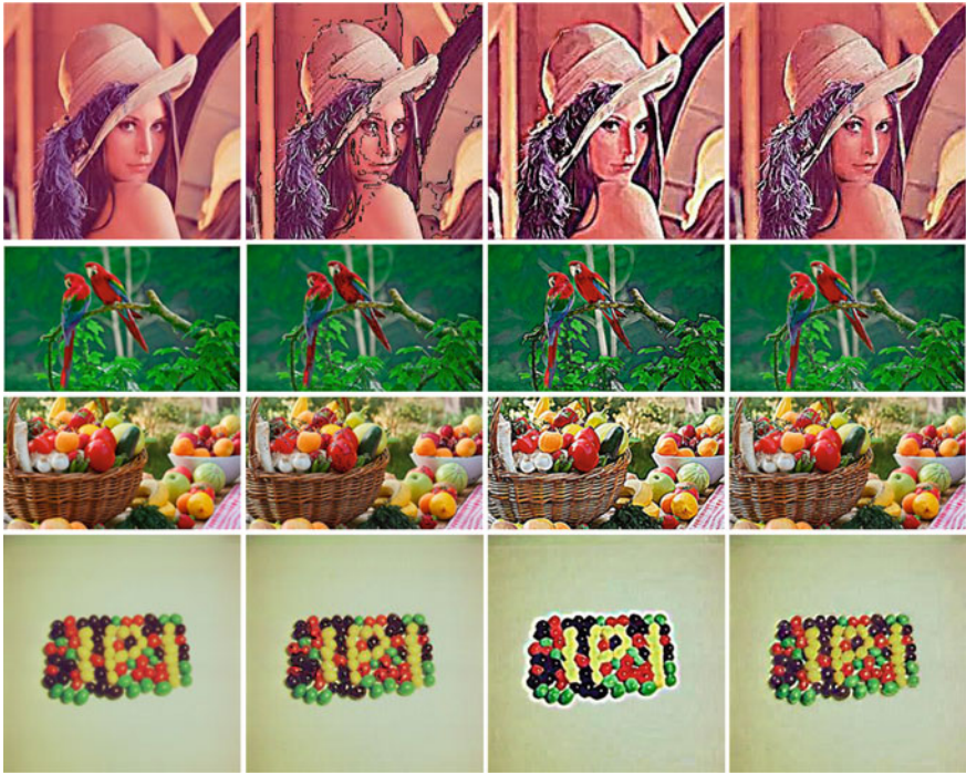
Fig. 4 Contrast enhancement results for different test images, first column: original color images, second column: results with marginal ordering, third column: results with distance-based vectorial ordering, and fourth column: results of proposed Hilbert space filling curve-based mapping
