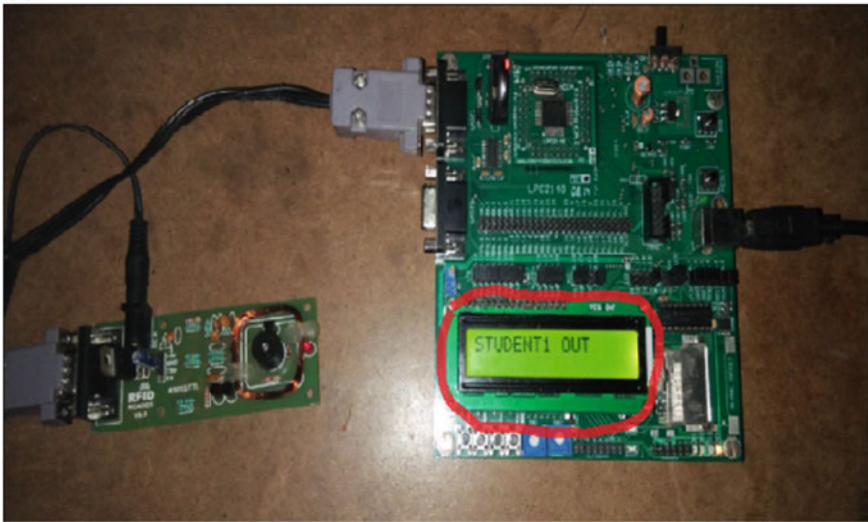
Fig. 3 a Interfacing RFID reader and LPC2148 b Student 1 exit status
