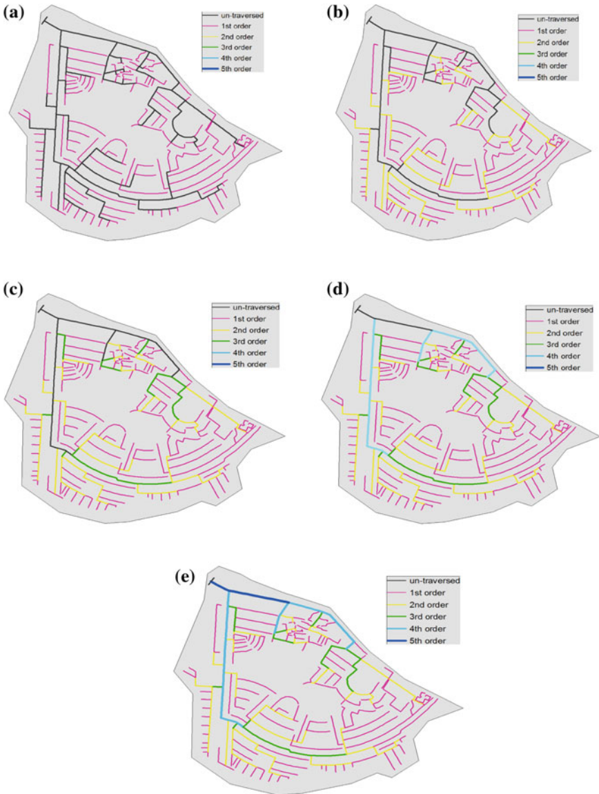
Fig. 6 a Network traversal after first-level ordering. b Network traversal after second-level ordering. c Network traversal after third-level ordering. d Network traversal after fourth-level ordering. e Network traversal after fifth-level ordering
