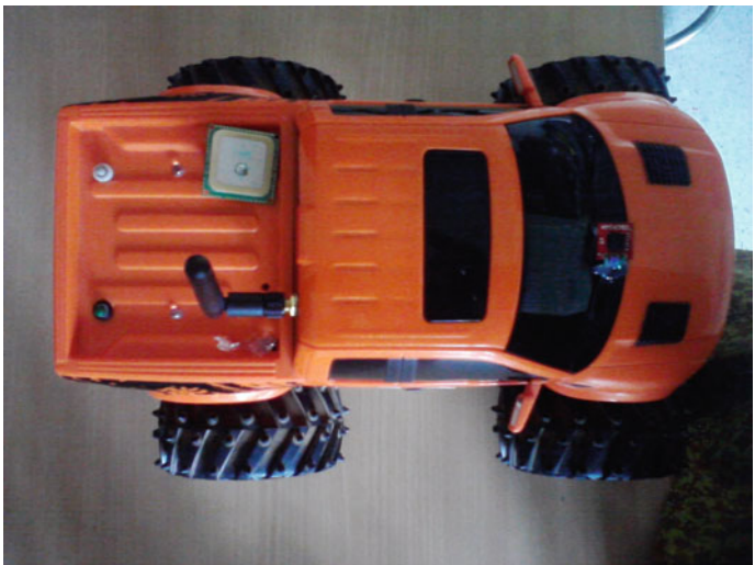
Fig. 7 Prototype fitted with GPS, Xbee and compass module
