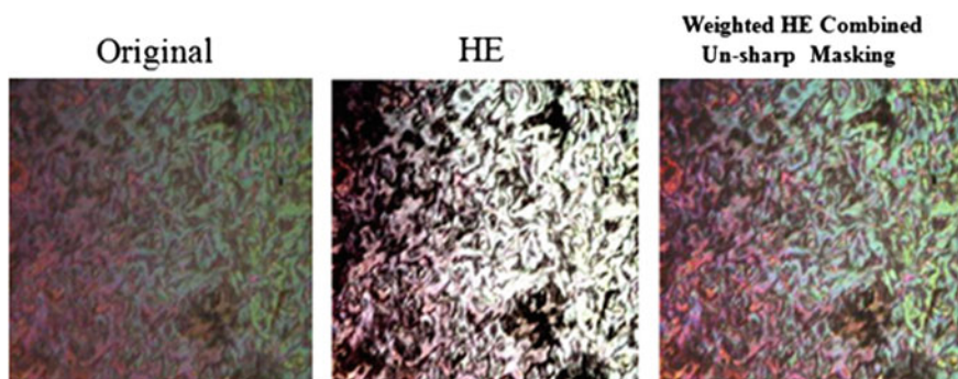
Fig. 7 Nematic transition in 1% ZnO nanodispersed 100.O6 compound at 109.5 °C
