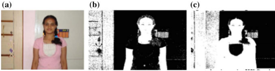
Fig. 1 a Input image, b segmented region using HIS color model, c segmented region using YCbCr model
