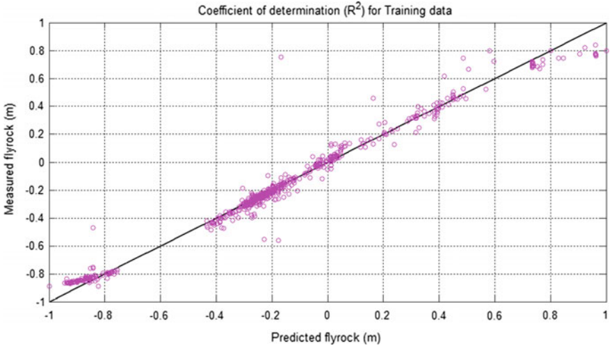
Fig. 2 Fly-rock distance versus predicted fly-rock distance in meters according to ANN testing data
