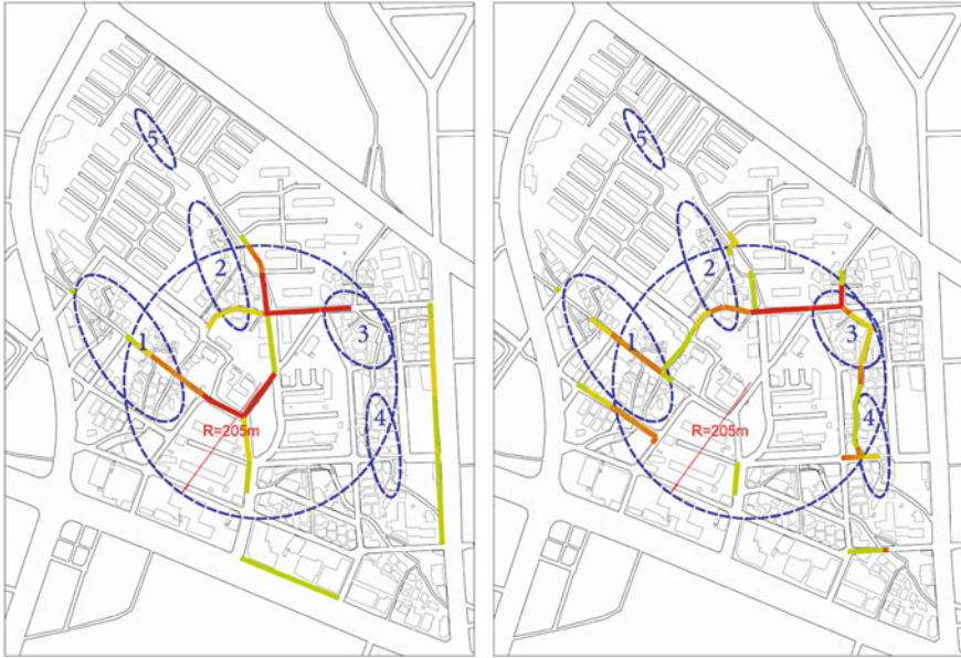
Fig. 7 Angular choice metric R_n (left) and R_{220} (right); streets with higher values were presented
