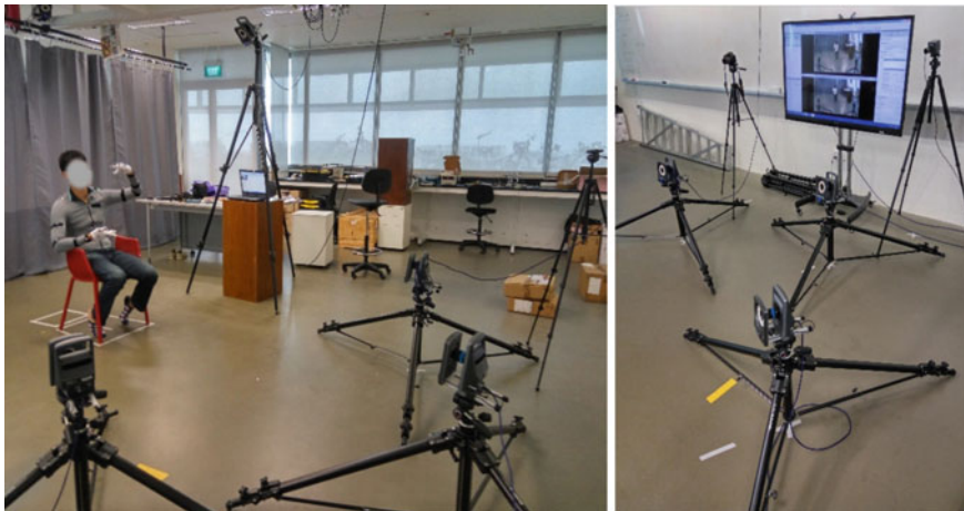
Fig. 3 The Vicon motion capture system setup design for the experiment
