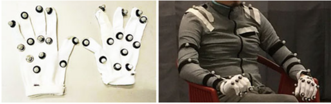
Fig. 1 Gloves and jacket with reflective markers worn by subjects during the experiment
