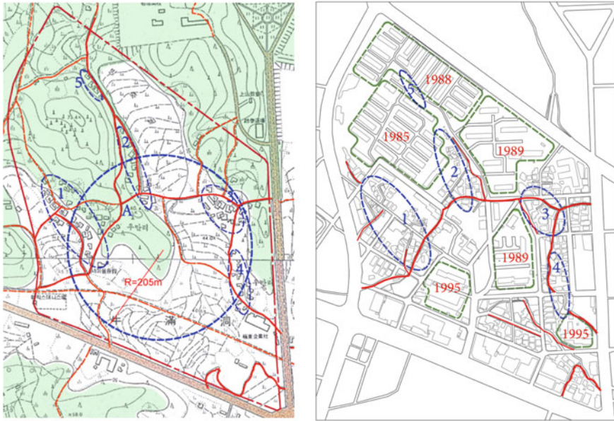
Fig. 2 Wooman old map (left) with rural roads (red and orange); and current map (right) with remaining traces of the old roads (red) and new apartment developments (green boundaries)
