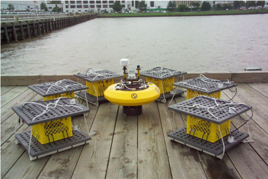
Fig. 8 Sediment microbial fuel cell called benthic unattended generator (BUG)
