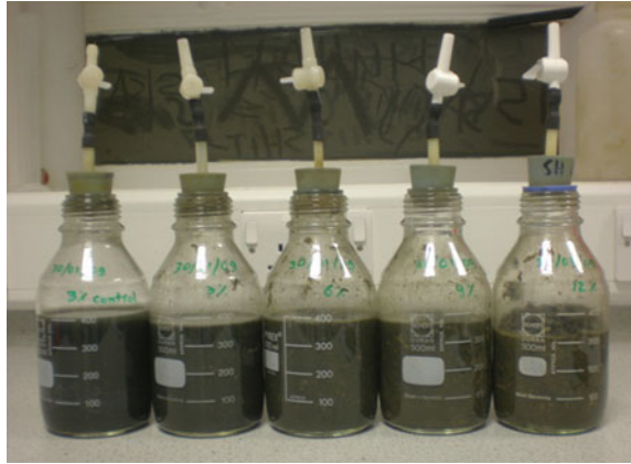
Fig. 5 Laboratory scale 400 mL anaerobic reactors used in BMP testing [9]
