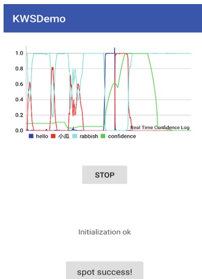
Fig. 5. Screenshot of the Android APP for wake-up word detection. (Color figure online)
