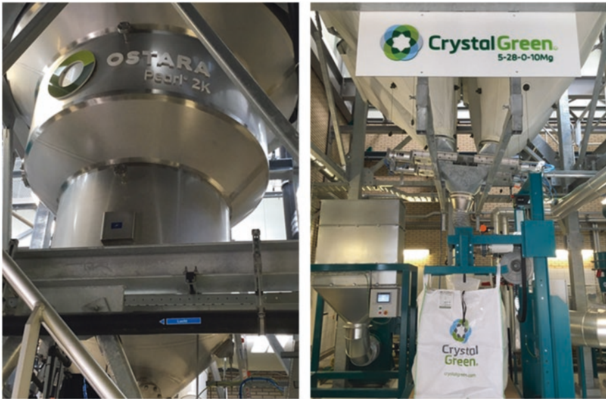
Fig. 3.4 PEARL struvite recovery reactor and Crystal Green bagging station in Amersfoort (source: Kabbe)
