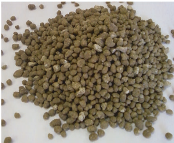
Fig. 16.6 PK 8-27+7MgO from plant-scale test with Airprex struvite
