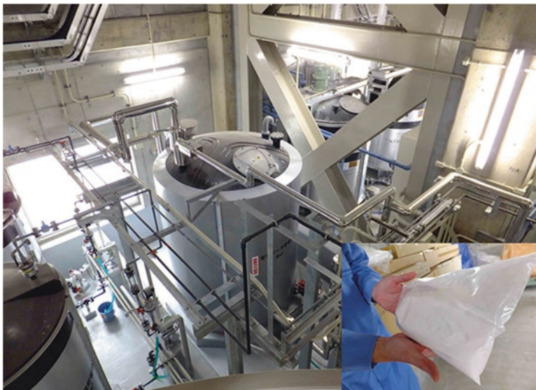
Fig. 1.3 Full-scale plant for recovering P from SSA at Tottori WWTP ( inset , recovered P product, HAP) (Photograph courtesy of M. Hashimoto)
