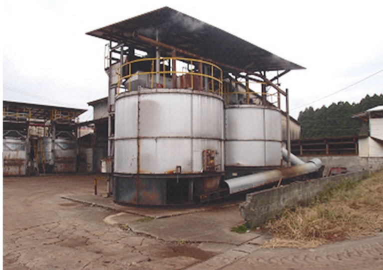
Fig. 25.2 Vertical aerobic fermentation
