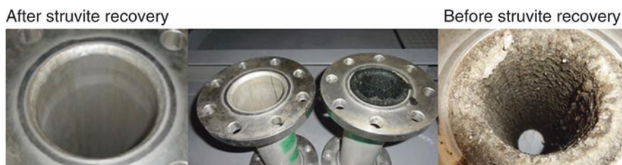
Fig. 17.11 The effect of struvite recovery on the scale buildup in pipe lines
