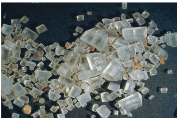
Fig. 16.5 Struvite crystals from the Airprex process (STOWA 2012)
