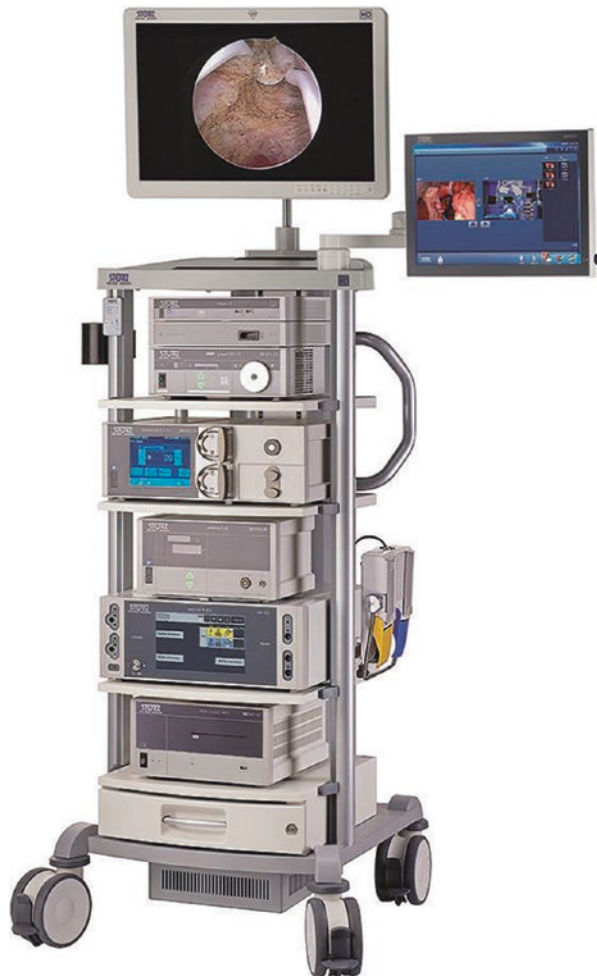
Fig. 1.1 Equipment cart for hysteroscopy, camera system, monitor, light source, fluid management device, electrocautery unit, and documentation system (Courtesy: Karl Storz)
