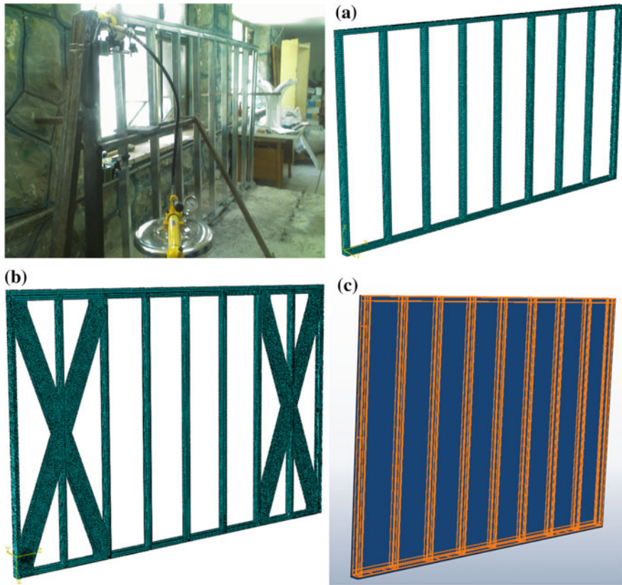
Fig. 6 a Laboratorial and FE models of first specimen: Frame without bracing but with semi-rigid connections b second specimen: Frame with X-shaped bracing and with semi-rigid connections and c third specimen: Frame without brace but in-filled with lightweight concrete
