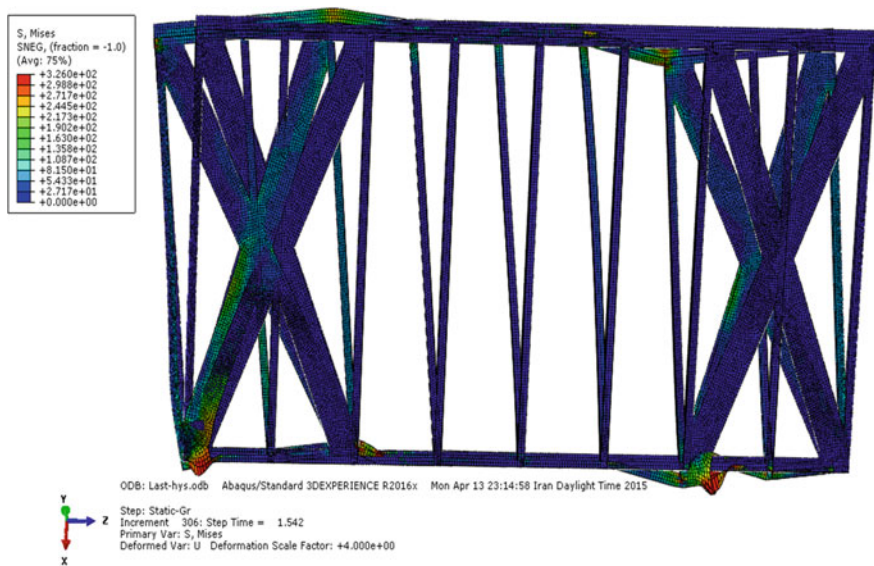
Fig. 11 Buckling of braces and sinus shape of deformation in second specimen
