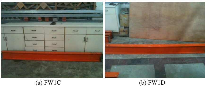
Fig. 4 Deformed FW sections after failure
