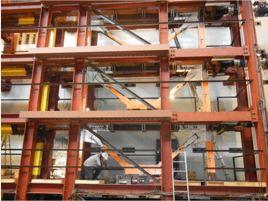
Fig. 4 Viscous damper usage in shear wall
