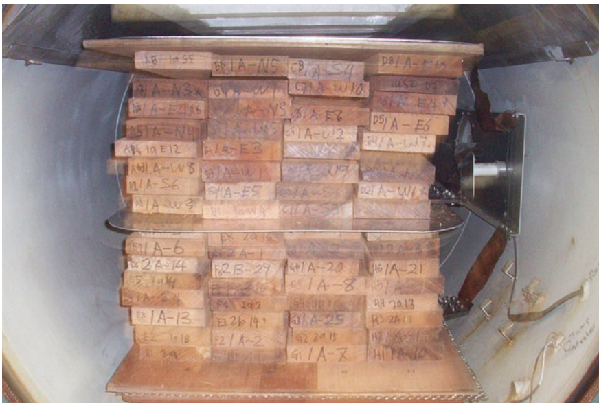
Fig. 1 Stacking of the timber samples in the RFV chamber
