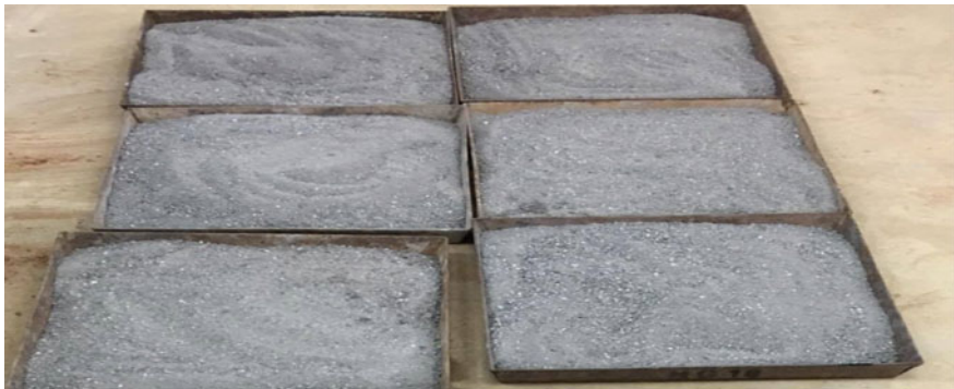
Fig. 2 Untreated marine clay sieved to 2 mm size
