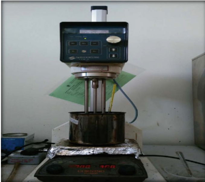
Fig. 1 Binder blending with shear mixer
