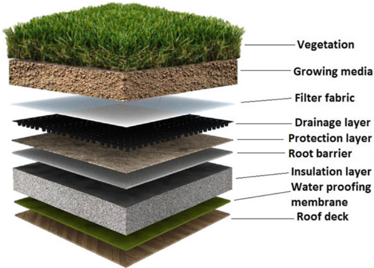
Fig. 1 Components of green roof [36]
