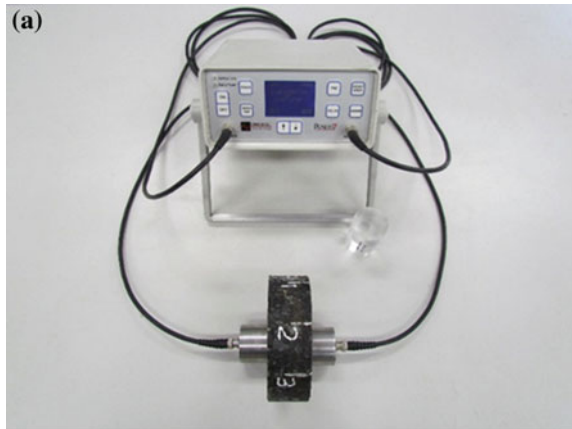
Fig. 2 a Pundit 7 with two 50 mm transducers. b Test locations for ultrasonic measurements
