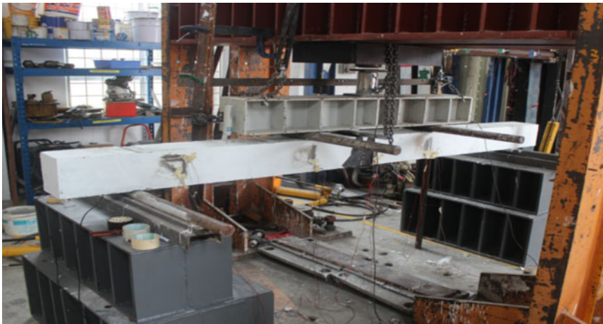
Fig. 4 RC grade 50 test setup
