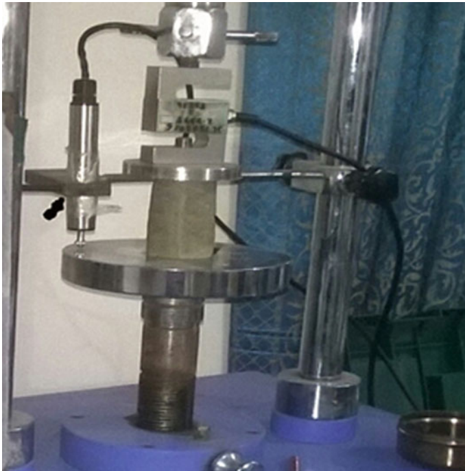
Fig. 6 Unconfined compressive strength test set up
