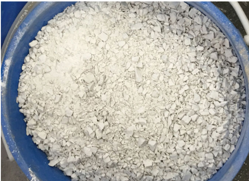
Fig. 3 RBT crushed into 5 mm using the crushing machine
