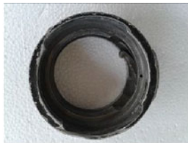
b. Ratchet buckle failure
