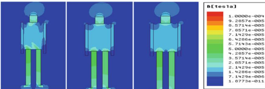
Fig. 5 Distribution of magnetic field intensity around human body
