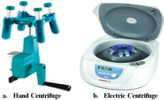
Fig. 2 Types of centrifuge: (a) hand centrifuge; (b) electric centrifuge
