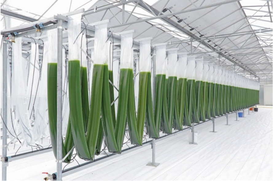
Fig. 6 Bag photobioreactor. (Source: https://www.pinterest.co.kr/pin/530791506060698316 )
