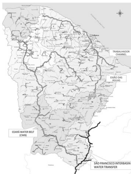
Fig. 10.10 Strategic water infrastructure of Ceará State: Worker's Channel (1993), Integration Channel (2012), São Francisco River Transfer Project integration (scheduled for 2018), and Ceará Water Belt (under construction). Source SRH-CE (2017a)
