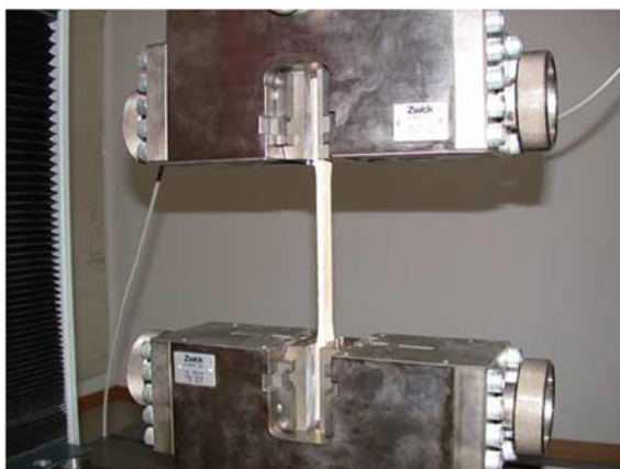
Fig. 3 Uniaxial stretching test setup. The white tissue testing strip (center) is mounted between two holders (above and below) and is being elongated by them. The force applied and the resulting elongation are monitored simultaneously and plotted as force versus elongation curves [15, 54]
