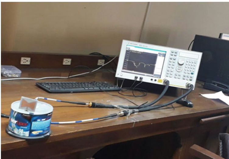
Fig. 8 Practical setup to measure return loss of proposed antenna at IIT Kanpur
