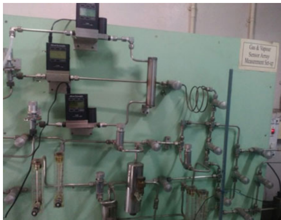
Fig. 2 Experimental setup for ZnO-based thin film gas sensor for detection of H 2 gas
