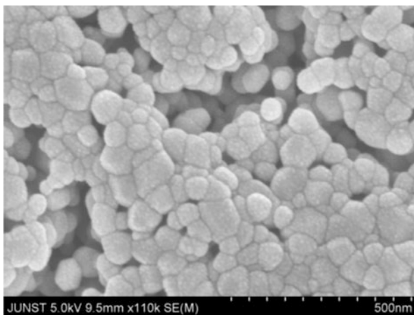
Fig. 5 FESEM picture of Pd/n-ZnO thin film sensor at operating temperature 350 °C
