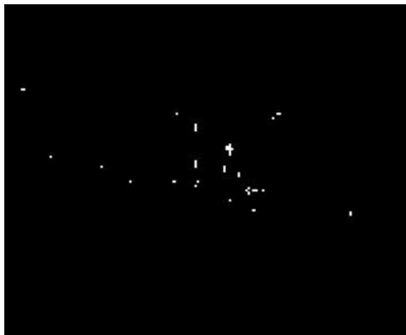
Fig. 6 Binary image of background subtracted frame I_{diff}
