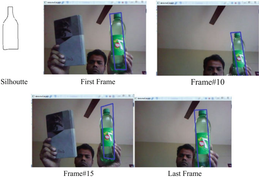
Fig. 13 Results of bottle tracking in the presence of book movement in different frames
