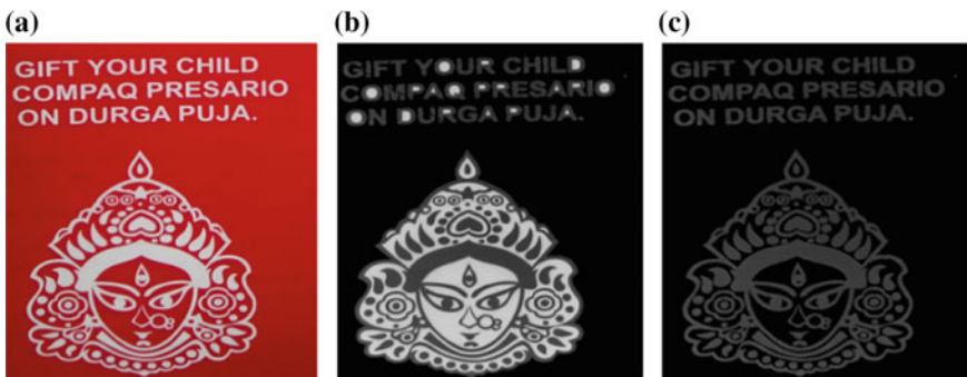
Fig. 2 Effect of region growing algorithm with varying number of seeds. a Sample image, b image with background suppression for single seed point, c image with background suppression for multiple seed points
