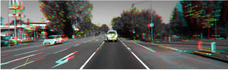
Fig. 1 Feature selection without grid-based feature selection
