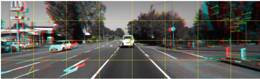
Fig. 2 Feature selection with grid-based feature selection
