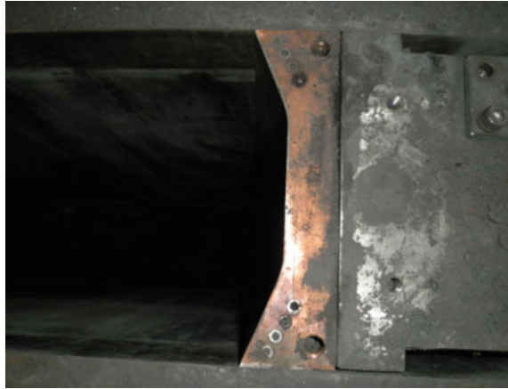
Fig. 13 The photo of the chamfered mould applied in industrial production
