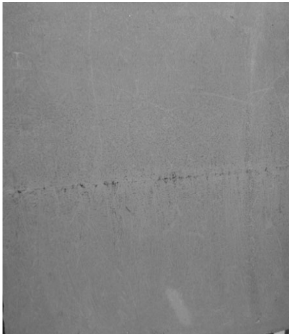
Fig. 3 Macrostructure of thick slab (300 mm) with soft reduction
