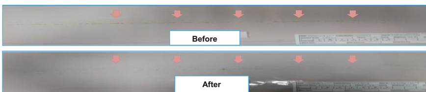
Fig. 11 Centre line segregation before and after improved cooling strategy
