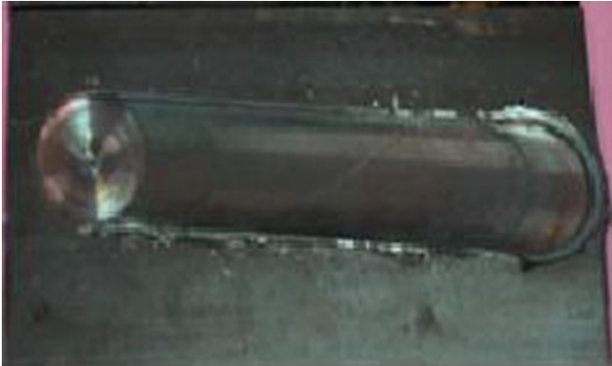
Fig. 1 Bead-on-plate FSW weld at 80 rpm
