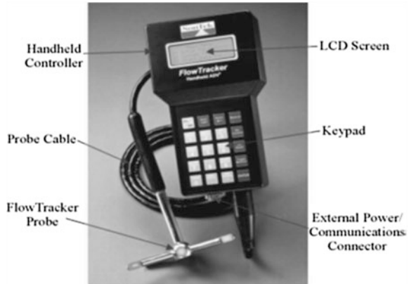
Fig. 2 Flow Tracker with 2D probe principle of operation
