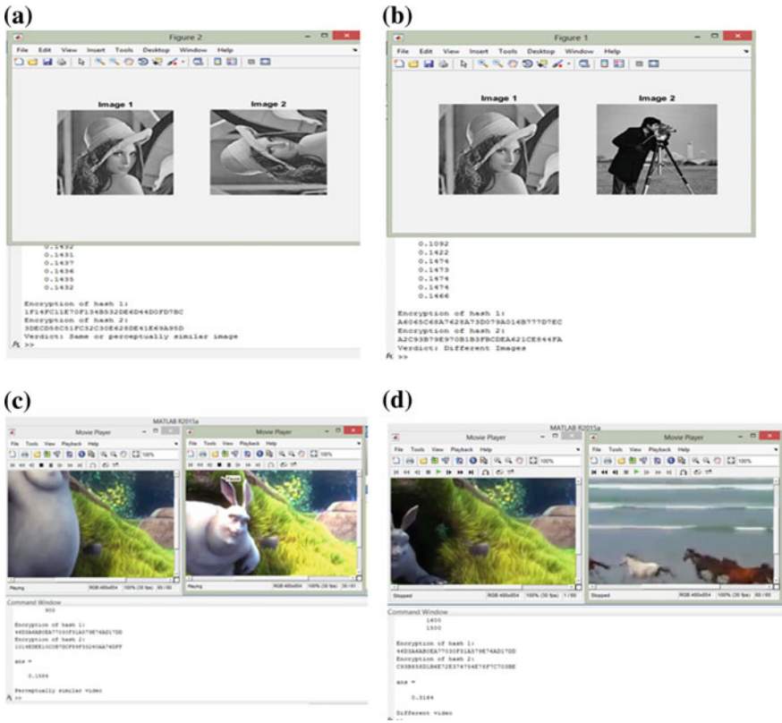
Fig. 3 pHash for images and videos is generated, and the hash values are encrypted and calculation of hamming distance is calculated to determine whether the data are the same (perceptually similar images/video) or different data
