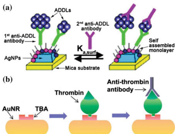
Fig. 5.2 Schematic representations of LSPR sensors based on a antibody–antibody sandwich assay. Surface-confined AgNPs were firstly synthesized on mica substrates. Next, the first anti-ADDL antibody was covalently attached to the AgNPs which have been passivated for nonspecific binding and activated for the attachment of antibody by the self-assembled monolayer. After incubated in varying concentrations of ADDLs, the samples were incubated in the second anti-ADDL antibody solution to enhance the LSPR shift response of the ADDLs (Reprinted with permission from Ref. [25]. Copyright 2005 American Chemical Society); b antibody–aptamer sandwich assay. TBA-modified AuNRs were incubated with thrombin to trigger thrombin bind to the AuNRs. The thrombin binding event generated a LSPR shift, which was amplified by the incubation of the thrombin-bound AuNRs in a solution containing anti-thrombin antibodies. The binding of anti-thrombin to thrombin caused further local refractive index changes at the AuNR surface, generating secondary redshift of LSPR peak (Reprinted with permission from Ref. [26]. Copyright 2012 Elsevier)
