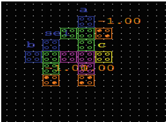
Fig. 6 Layout of 2:1 multiplexer in QCAD
