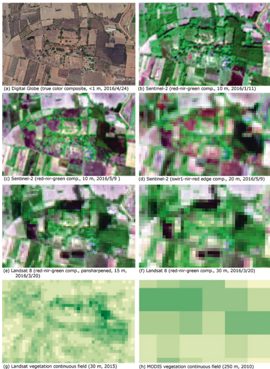
Fig. 5.1 How are TOF picked up by remote sensing products with different spectral and spatial resolutions? All panels show the same piece of land located approx. 25 km north of Bangalore, India (central coordinate: WGS84, UTM 43P 780200 E, 1466350 N), at about the same date and, if possible, using the same combination of spectral bands. The depicted area contains a diverse mixture of agricultural fields, single trees, tree groups, tree plantations, and built-up structures. Panel (a) shows a high-resolution image (Google, Digital Globe) downloaded via Google Earth in which most TOF features can easily be distinguished from other land cover by the human eye. In
