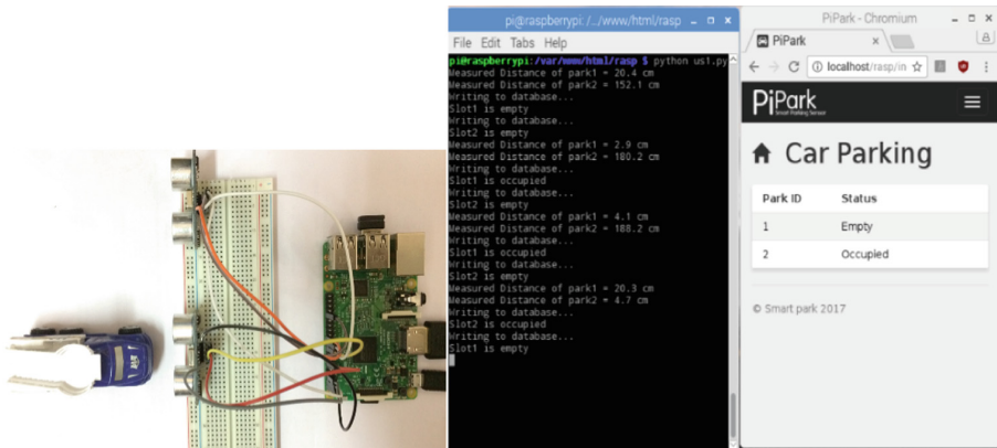
Fig. 5. Connection and output when first slot is empty and second slot is occupied
