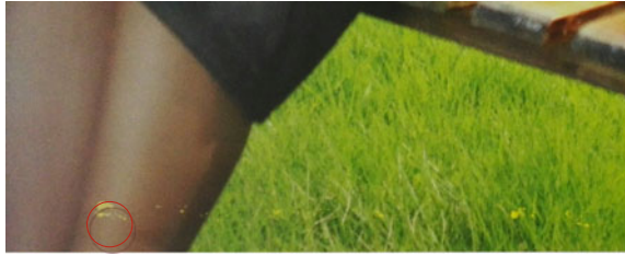
Fig. 3 Ink on the surface of the printing sheet
