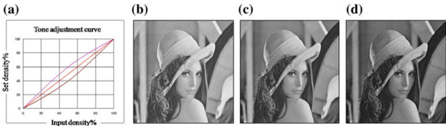
Fig. 4 Evaluation of image: a density control curve, b density reduction portrait, c original image, d density increase portrait
