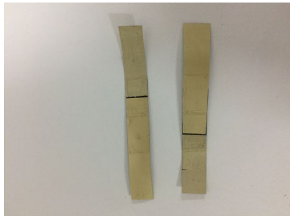
Fig. 2 Samples of homemade flexible pressure sensor
