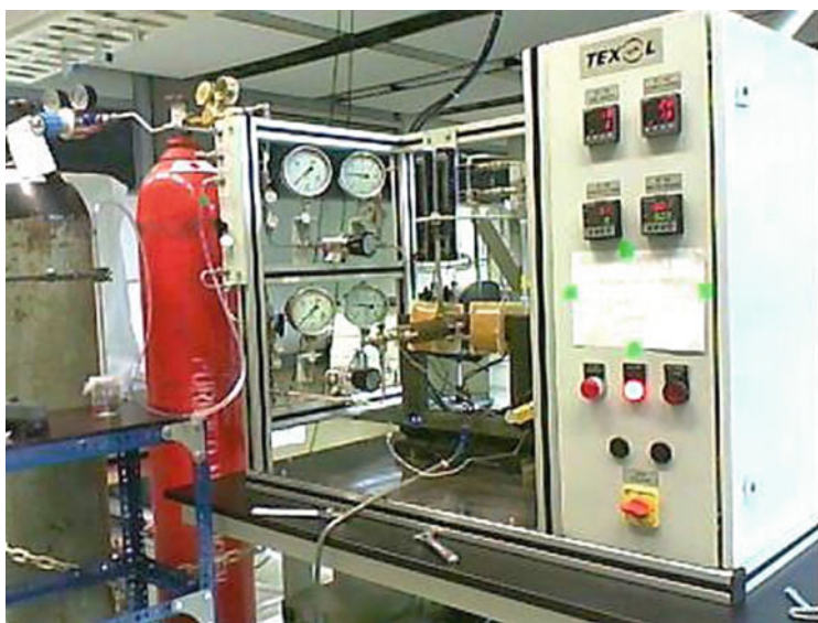
Fig. 3.5 First version of the lab-scale novel ammonia synthesis system
