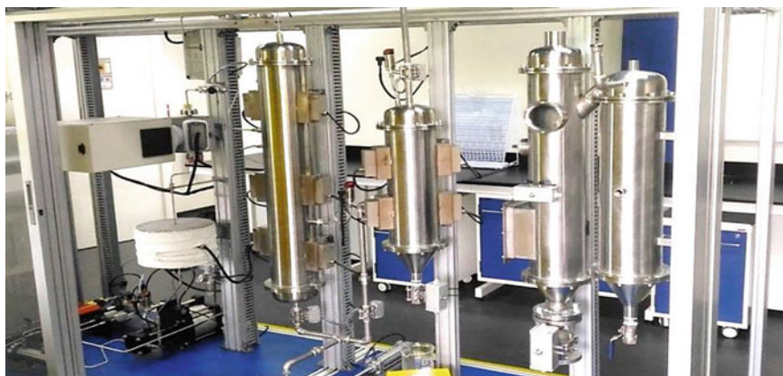
Fig. 3.13 Experimental setup of pilot-scale green urea reactor
