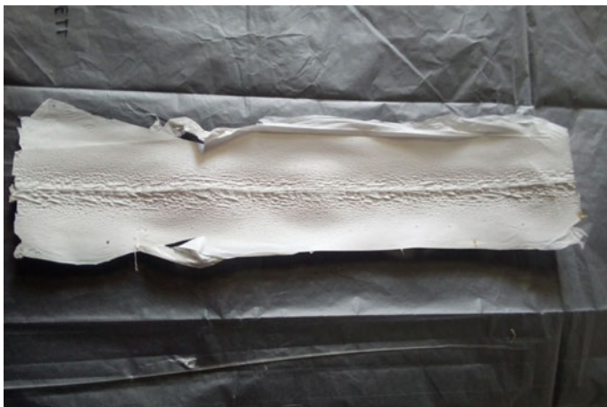
Fig. 1 Electrospun membrane of CaO from egg shells
