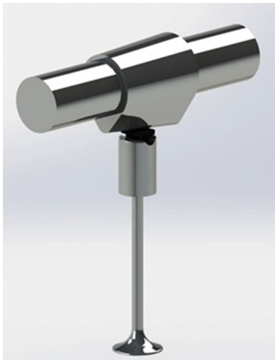
Fig. 10 Schematic of a three-dimensional cam lobe system
