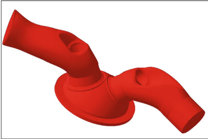
Fig. 12 Final design of intake and exhaust manifold
