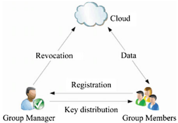
Fig. 4 Distributed key process between different users in TTKM procedure
