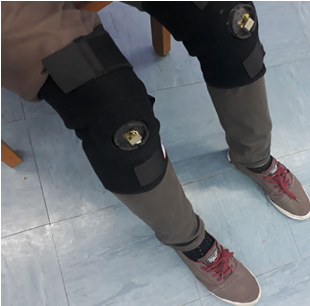
Fig. 2 3D printed sensor band and its placement on the knee
