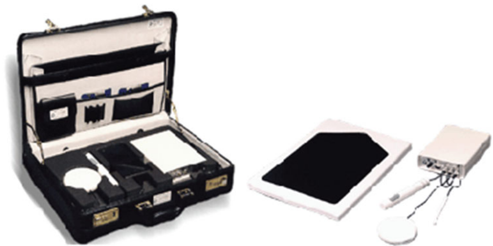
Fig. 1 A set of instruments in CATSYS system which consists of a data logger and four sensors, including a force plate for balancing measurement (static posturography), a reaction handle, a touch recording plate and a tremor pen [22]
