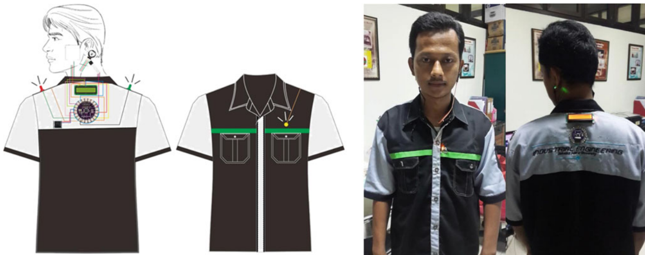
Fig. 3 Illustration of thermal and heart rate monitoring circuit system which was installed on the clothing
